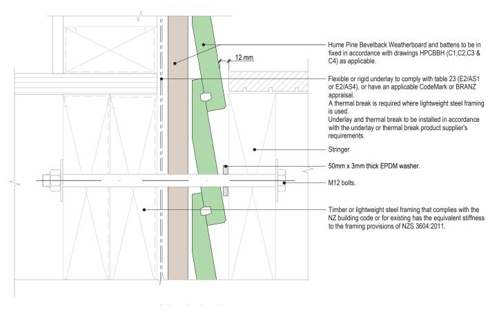
Hume Pine Bevelback Weatherboard Non-cantilevered Deck Junction
